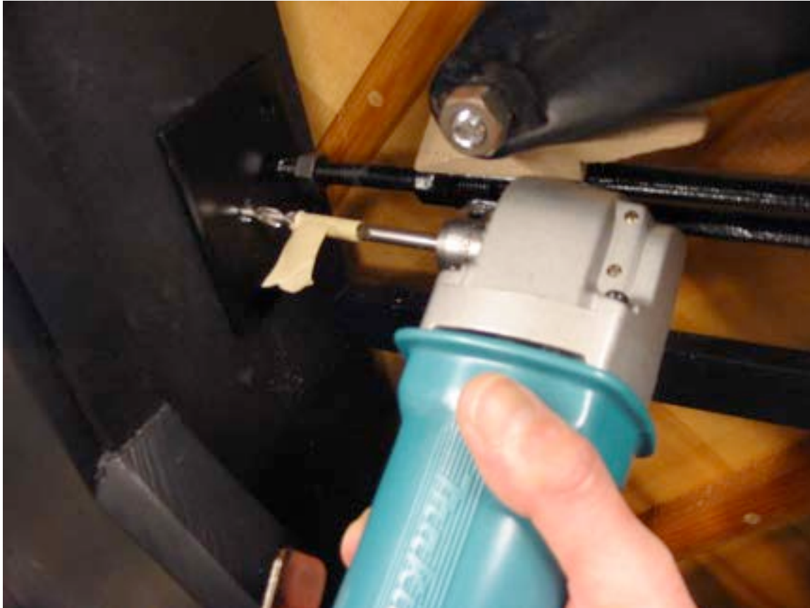
Photo 6 Drilling the first hole in the belly rail for the Belly Plate
