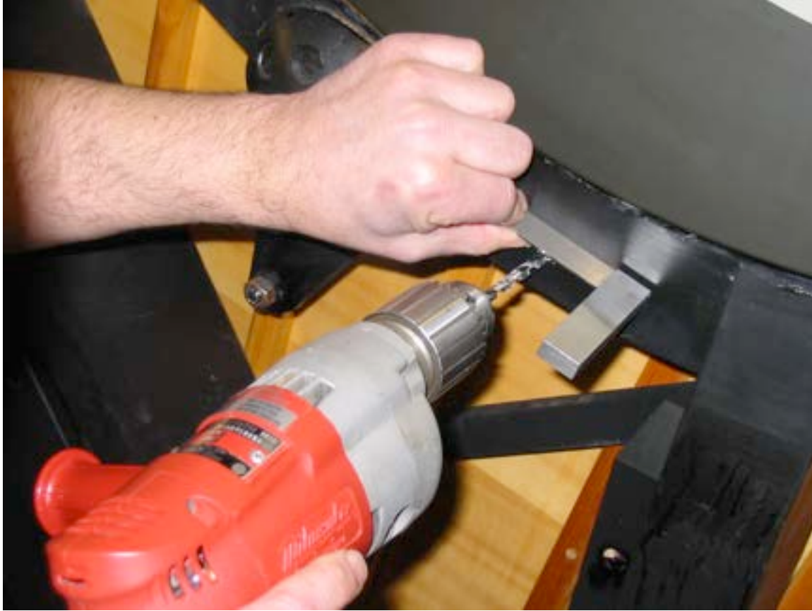
Photo 3 Aligning the drill with the use of a machinist square
