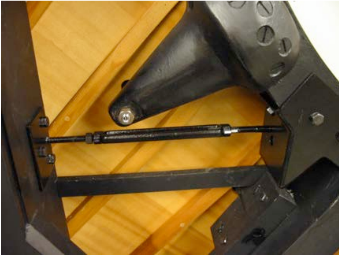
Photo 8. Completed installation of the Treble Resonator
