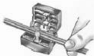
Place wire from heater bar in groove. Be sure it lies flat without twist.
