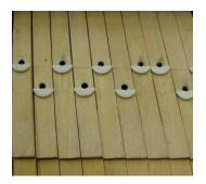
Many times we come across piano actions that have a heavy touch weight, even with friction at an acceptable 10-12 grams (downweight minus upweight divided by 2). This can be caused by installing new hammers that weigh more than the original, without leading the keyboard.
