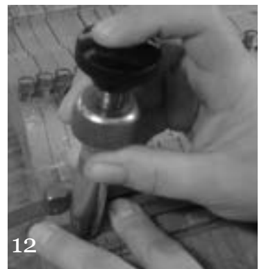
Continue to lightly hold felt with fingers and press plunger to cut.
