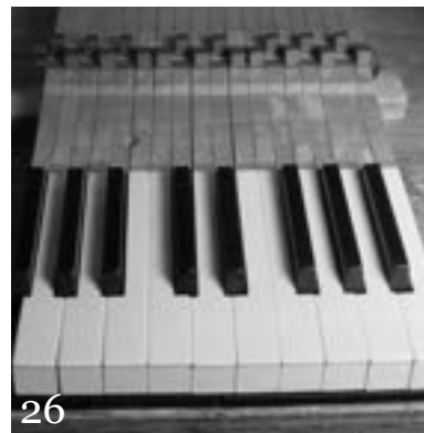
Trimming cloth. As before, use finger to hold caul while cutting.
