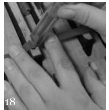
With glue in sharp mortises, lay felt across and cut same as balance rail.
