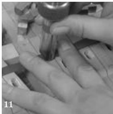
Insert Bushmaster into mortise and hold cloth with fingers.
