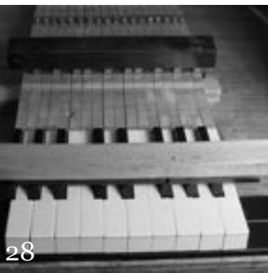
Position "clamp" over sharp rail.
