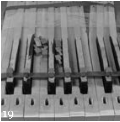
Sharp rail completed. Trim rail before bushing naturals.
