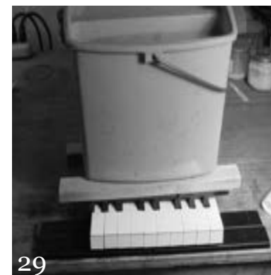
Add weight for clamping sharp rail and counter weight for front clamps.
