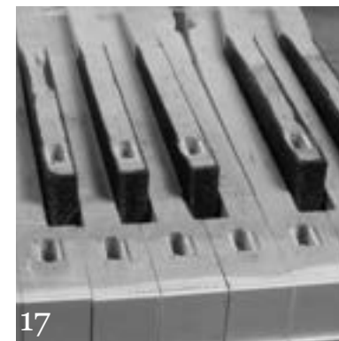
Push naturals away from sharps. Tape will still hold the section together.
