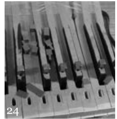
Completed sharp rail.
