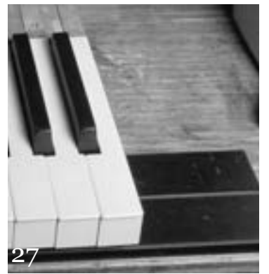
Rest cauls on hard rubber and make sure cauls are straight.
