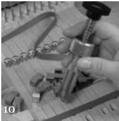
With glue in all the sharp mortises, lay the cloth strip over the mortises.
