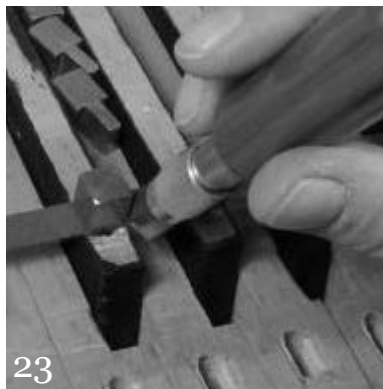
Trimming cloth. As before, use finger to hold caul while cutting.
